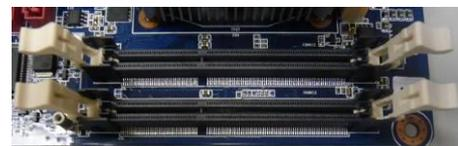
204-pin DDR3 SO-DIMM sockets
