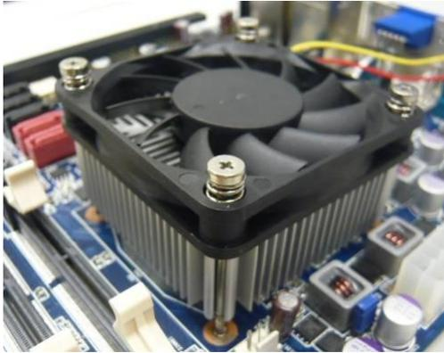
3. Screw tightly the four fasteners.
